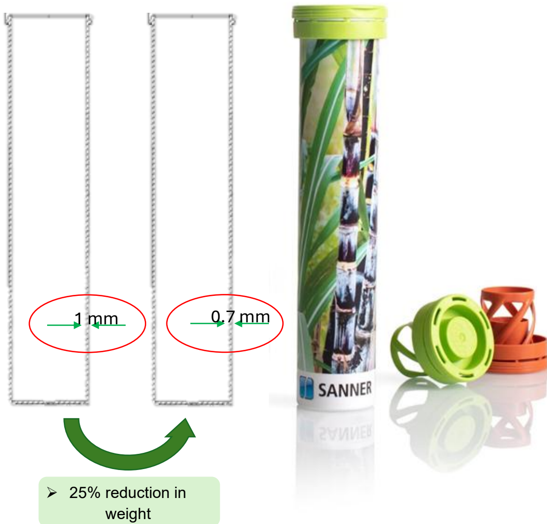
Fig.14 Possible material reduction for an effervescent tablet tube by reducing the wall thickness of the tube
