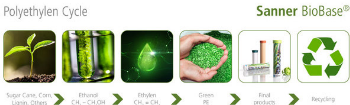
Fig. 2: The life cycle of bio-based polyethylene (© Sanner GmbH)
